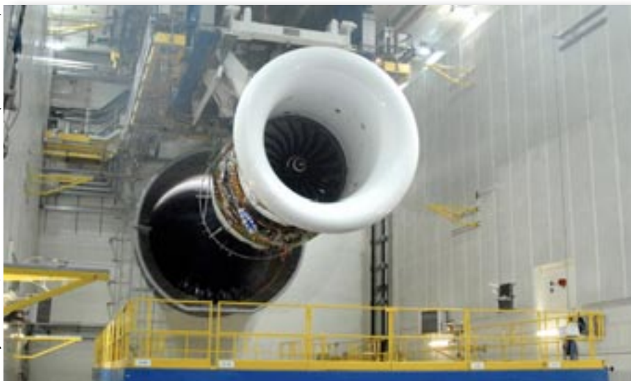
Trent turbofan under test at Rolls-Royce Derby, where it is currently testing UltraFan the next generation of efficient engine technology.
